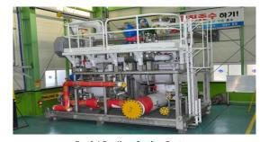
Partial Re-liquefaction System
