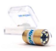
capsule captures images of the GI tract, which are sent via Human Body Communication to sensor pads which are affixed to the patient body. The sensor pads are connected to the receiver by the data cables. The image data is stored on the receiver for the duration of the patient procedure. After removing the receiver set from the patient body, the receiver is connected via USB to the Commercial PC and the image data is uploaded.
